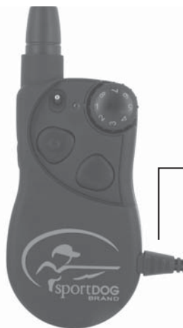
CHARGER CONNECTOR PLACED IN THE REMOTE TRANSMITTER CHARGING JACK
